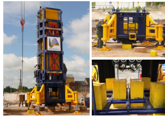
Fig. 19. StatRapid Load Testing Device and rubber cushioning system.
