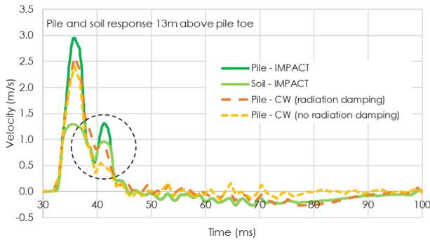
Fig. 11: Pile and soil velocity response.
