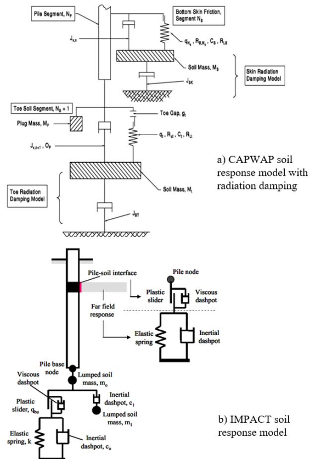
Fig. 9: Soil response models in CAPWAP and IMPACT, (a) PDI, 2006; b) Randolph, 2008.
