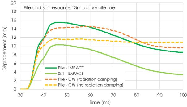
Fig. 10: Axial displacements.
