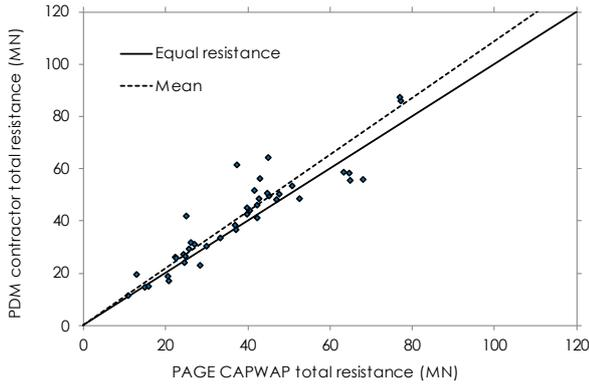
Fig. 8: Comparison of PAGE CAPWAP and PDM contractor total resistance from signal matching
