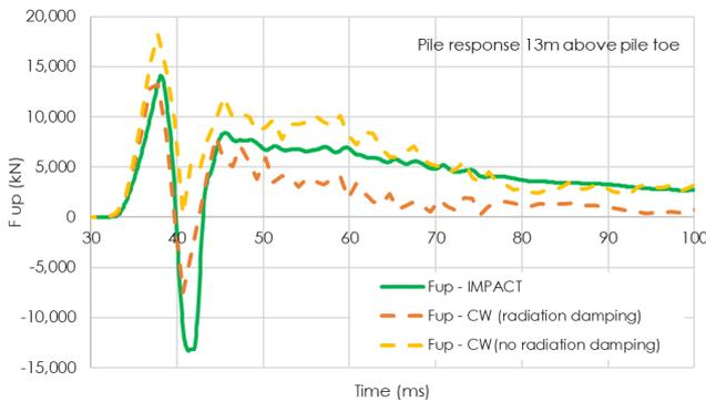
Figure 12: Upward traveling force wave
