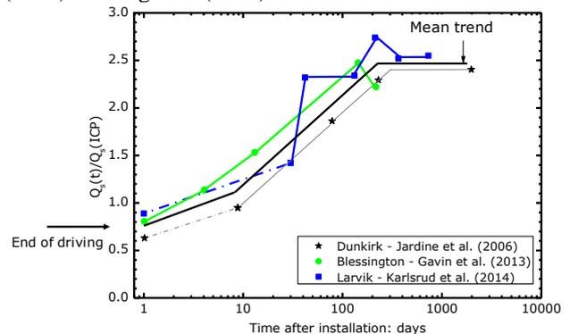
Fig. 2: Trends for growth in first-time shaft capacity with time at three sites, tension capacities normalised by pile specific ICP-05 predictions; after Rimoy et al. (2015).
