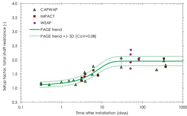
Fig. 21: Development of PAGE offshore piles' shaft resistances setup with time.
