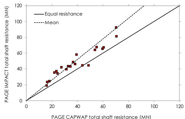
Fig. 6: Comparison of CAPWAP and IMPACT shaft resistance from signal matching.
