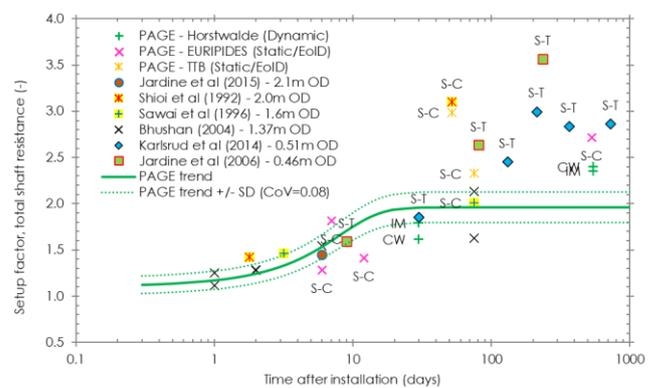
Notes: 1) S-T and S-C refer to setup based on EoD interpreted shaft resistance combined with tension or compression shaft resistance, respectively, from static tests after setup; 2) CW – CAPWAP, IM-IMPACT signal matching
