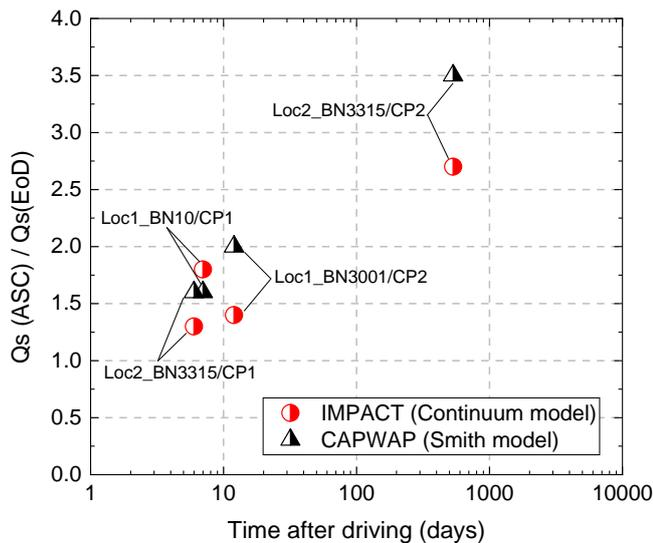
Fig. 17: Shaft setup  $Q_s(ASC)/Q_s(EoD)$  versus ageing days after driving from EURIPIDES pile tests.
