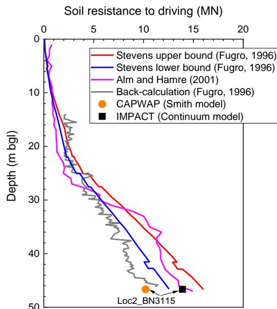
Fig. 16: Comparison between predicted and back-calculated soil resistance to driving: EURIPIDES, Location 2.
