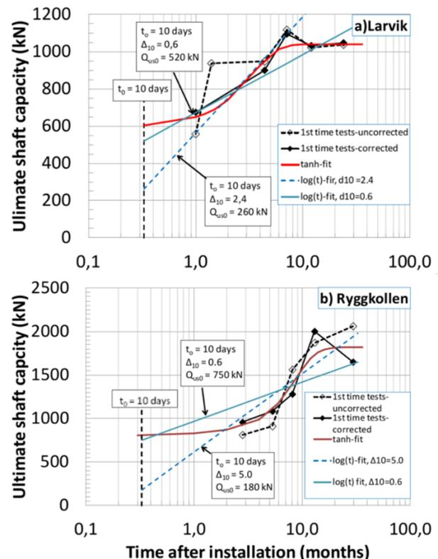
Fig. 4: Tension resistances at NGI test sites, Karlsrud et al, (2014)
