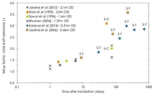
Note: S-T and S-C identifies cases in which setup was determined from static tension and compression tests, respectively, compared to EoID dynamic tests
