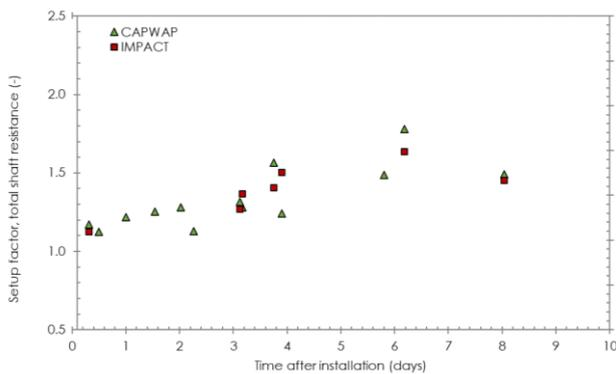
Fig. 22: Development of PAGE offshore piles' shaft resistance setup over first 10 days.
