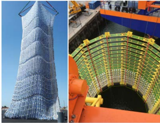
Fig. 11. (Left) The HSD system with a length of 40 m hanging from the crane. Source: https://www.offnoise-solutions.com/the-hydro-sound-dampersystem-hsd-system/ . (Right) The newly developed AdBm-NAS system showing the resonators in the array ( https://adbmtech.com/wp/ ) (Tsouvalas, 2020).
