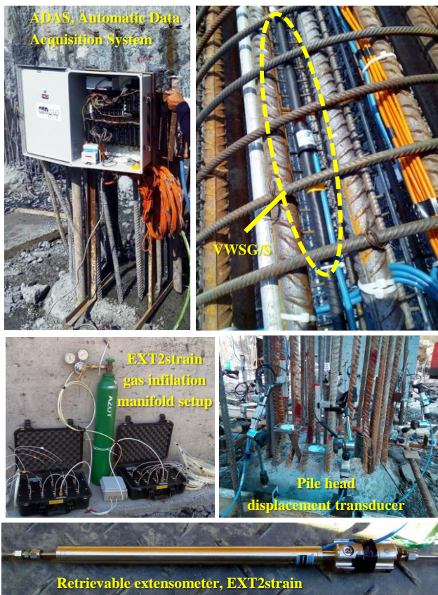
Fig. 3. General views from the instrumentation detail.
