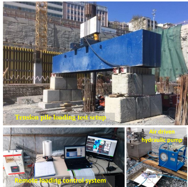
Fig. 6. General views from test setup, loading and measurement system.
