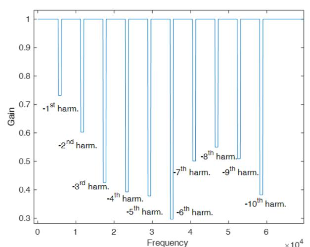
Window width for each harmonic increases due to spectral leakage
