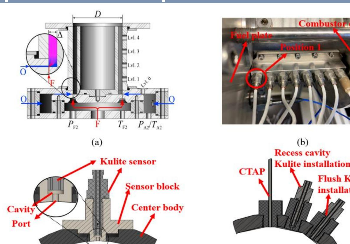
(a) TU Berlin's RDC, (b) recessed sensor block on the RDC, (c) cross section of a recessed mounted Kulite sensor, and (d) Kulite sensors in flush, recessed and CTAP configuration.
