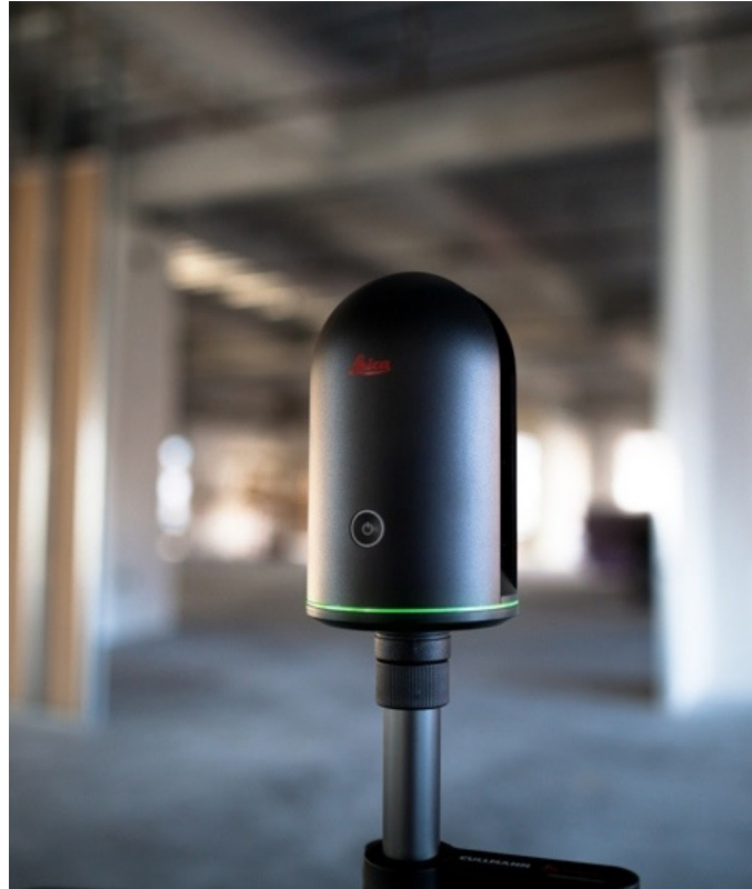
Figure 10 the BLK360 laser scanner - mounted on top of the robot
