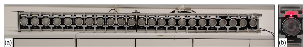
FIGURE 1 Experimental setup. (a) A horizontal array of 23 free-field speakers and 23 light emitting diodes (LEDs). (b) Detail of one speaker spatially aligned with one LED. In each trial, a single sound was simultaneously reproduced with a single red flash. Participants reported the auditory and visual stimulations as originating from exactly the same source
