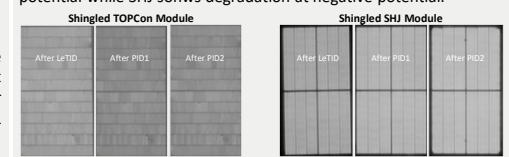
Figure 5 shows the relative degradation (top) and EL images (bottom) of the modules after PID with positiv firstly and negativ potential finally. TOPCon shows some degradation with both potential while SHJ shows degradation at negative potential.
