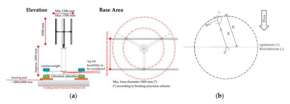
**Figure 1.** (a) Overall dimensions of the vertical axis wind turbine (VAWT) for rooftop installation;(b) schematic geometry of the passive variable geometry VAWT.
