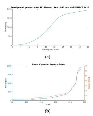
**Figure 2.** (a) Aerodynamic power for the VAWT rotor 1900 mm height, 850 mm maximum radius and turbine blades of NACA airfoil 4418 and (b) companion power converter look-up table to the VAWT rotor.
