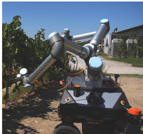
Fig. 1: Mobile bi-manual harvesting robot
