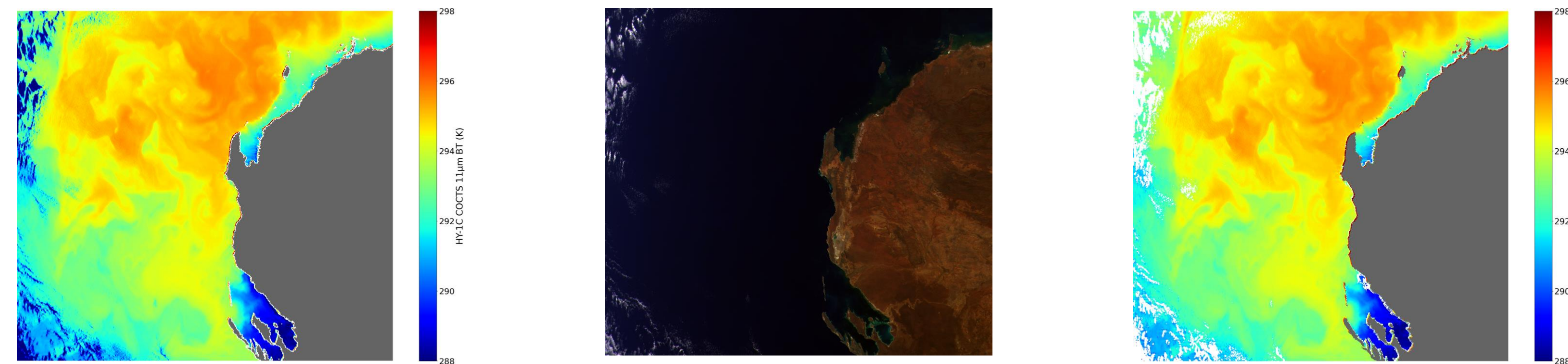
Fig. 1. Bayesian cloud detection results on 10 July, 2019: (a) COCTS 11 \mu\text{m} scene BT on before cloud detection; (b) RGB image of reflectance channels; COCTS 11 \mu\text{m} scene BT after cloud detection. The gray in (a) and (c) represents land and white in (c) represents cloudy sky.
