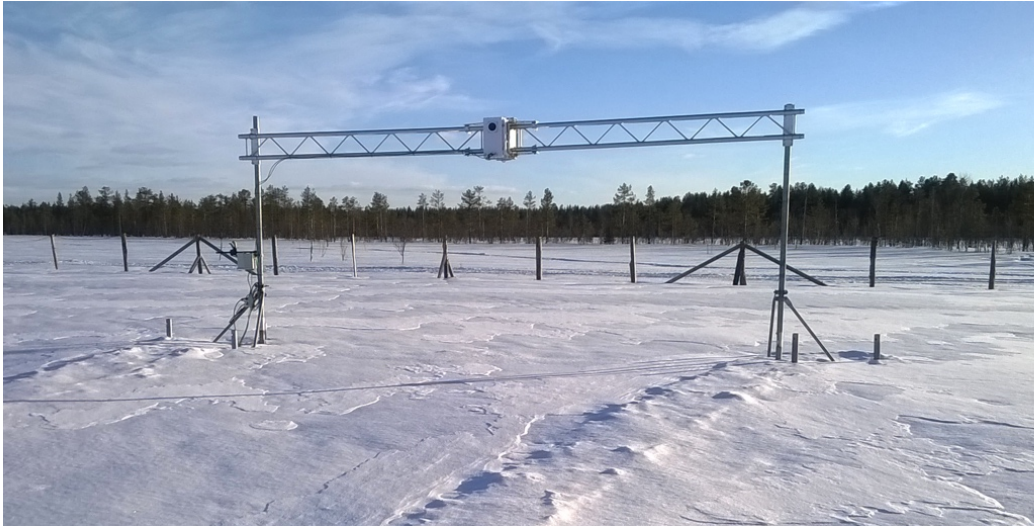
Figure 17: SVC-FMI spectro-albedometer installed in Sodankylä, Finnish Lapland.
