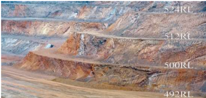
Fig. 6. Pit slope with initial 8 m high failure contained within a rock fall catchment bund on 26 October 2019–pit floor 492 RL
