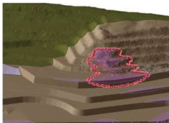
(b) FoS=1.20 for 48 m high multiple bench slope
