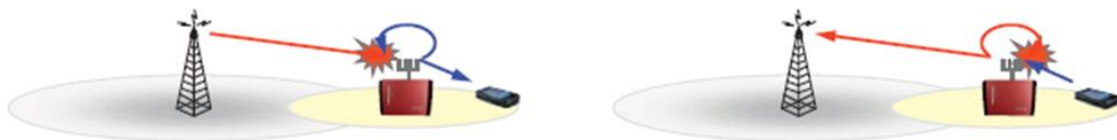
Figure 12. Interference between access and back-haul links [3]
