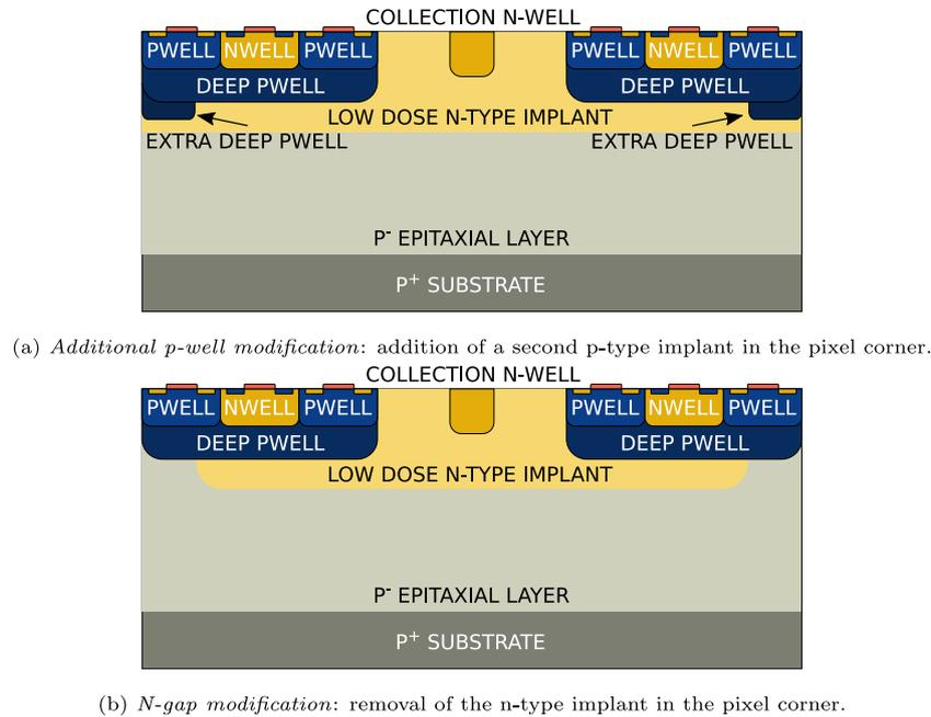
Fig. 2. Schematic cross-section of TJ-Monopix1 illustrating the modifications to the sensor to enhance the lateral electrical field in the pixel corners.
