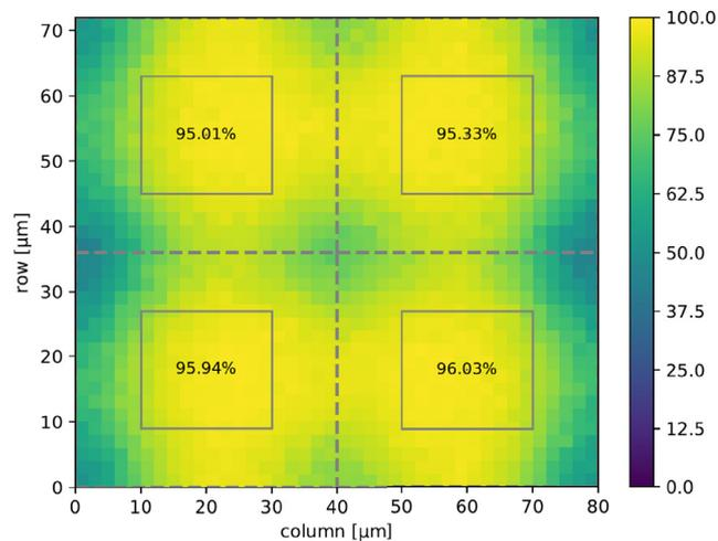
(a) Chip with 30  $\mu\text{m}$  thick sensitive volume at  $1 \times 10^{15} \text{ n}_{\text{eq}} \text{ cm}^{-2}$ .  $\epsilon_{Hit} = 87.1\%$
