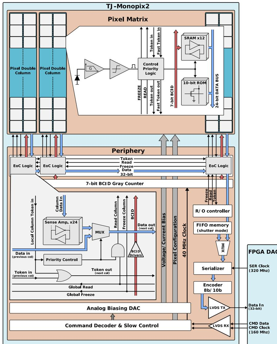
Fig. 3. Schematic overview of the digital logic in TJ-Monopix2 [9].
