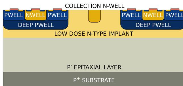
Fig. 1. Schematic cross-section of TJ-Monopix1 with a low-dose n-type silicon implant for a homogeneous electrical field and full depletion of the sensing volume (epitaxial layer).
