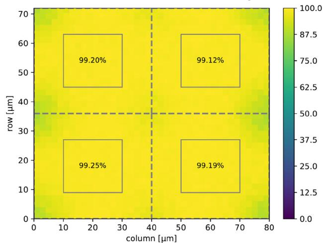
(b) Chip with 300  $\mu\text{m}$  thick sensitive volume at  $1 \times 10^{15} \text{ n}_{\text{eq}} \text{ cm}^{-2}$ .  $\epsilon_{Hit} = 98.6\%$
