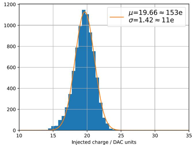
(a) Threshold distribution of an untuned TJ-Monopix2 chip.
