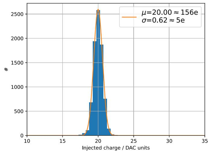
(b) Threshold distribution of a tuned TJ-Monopix2 chip.
