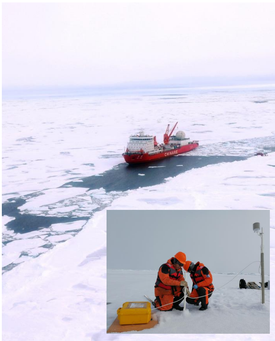
Figure 2.2.2. CHINARE2018 was implemented by R/V Xuelong ice breaker. The scientists are deploying SIMBA buoy on sea ice.
