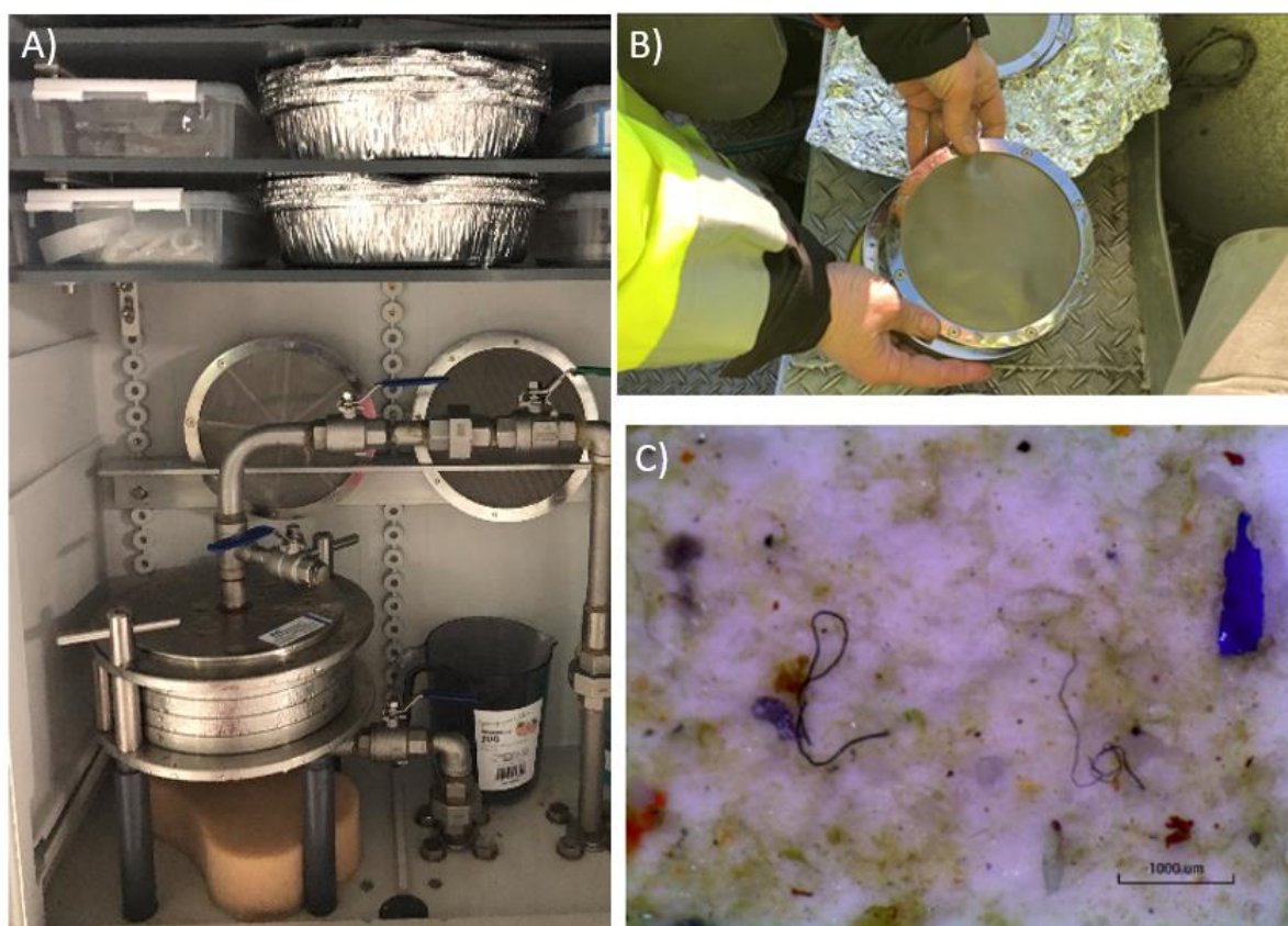
Figure 2.3.2. A) Photo of the INTAROS microplastics sampler equipped with three stacked filters in a dedicated FerryBox cabinet; B) Photo of a stainless steel filter (view from top) used to collect microplastics; C) Example of biological and abiotic material collected by the microplastics sampler; scale bar = 1000 µm.
