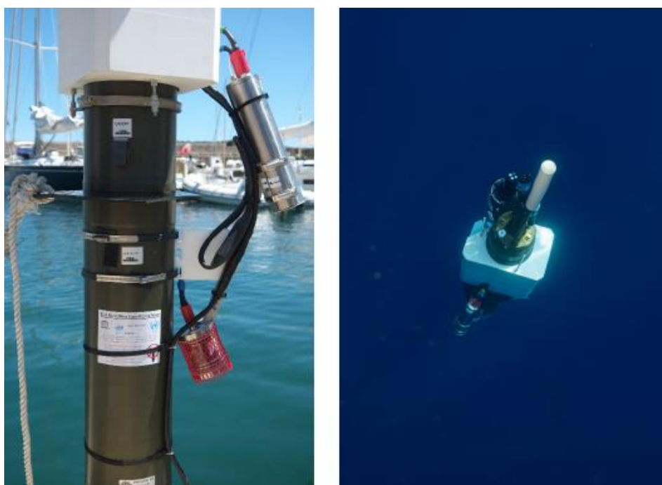
Figure 2.5.1. Proce float equipped with an UVP6, credit LOV.
