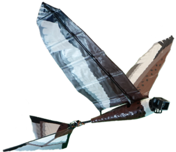
Fig. 1. GRIFFIN ornithopter prototype with fuselage and camera case in the head.
