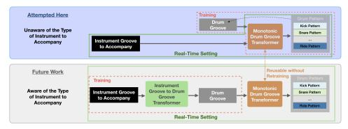
Figure 2: Instrument-unaware (top) vs instrument-aware (bottom) systems
