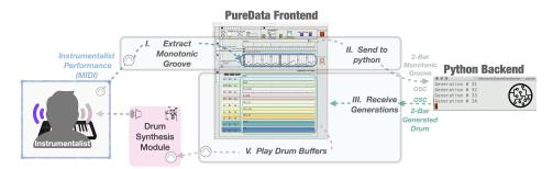
Figure 6: Overview of the developed real-time system
