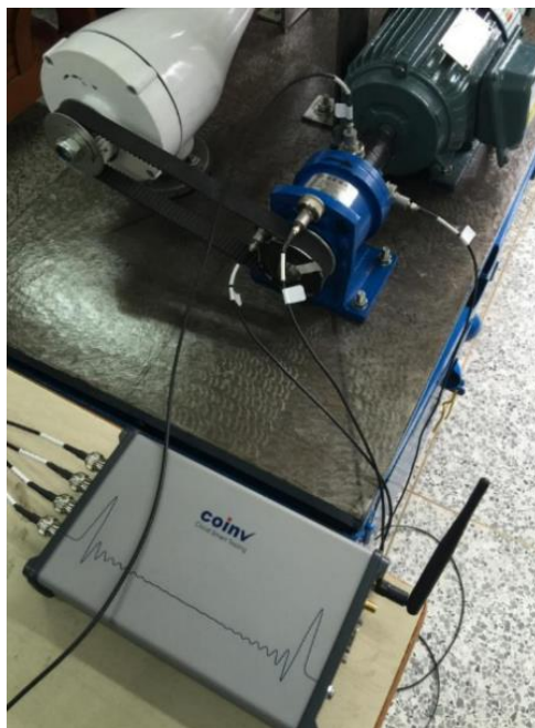
图5-3 振动信号的采集 Figure 5-2 Acquisition of vibration signals
