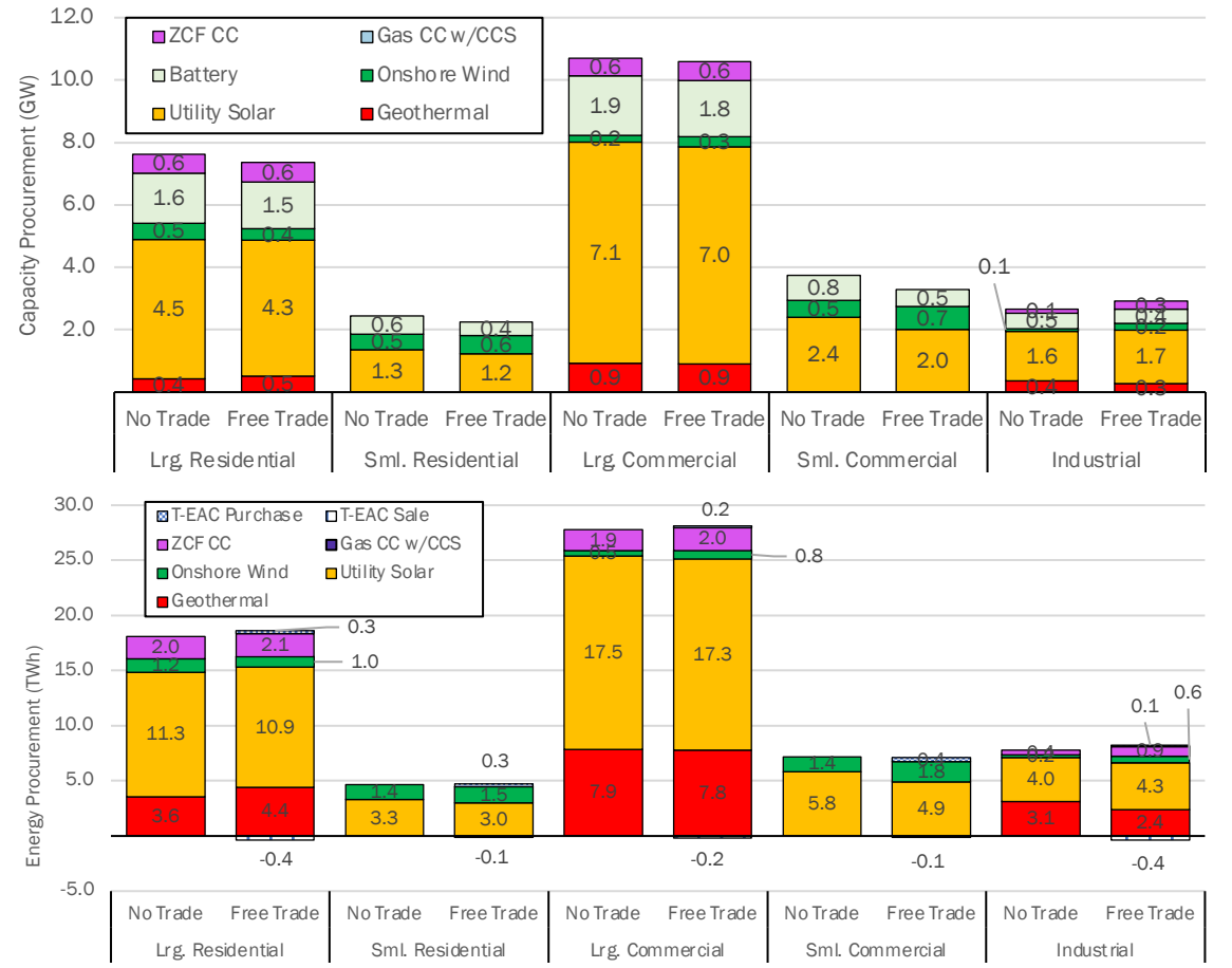
Figure A-2: Capacity and Energy Procurement of five modeled California participants, CFE score target = 98%, under the high natural gas price. High natural gas price makes NGCC with CCS much less economical, and the participants switch to combined cycle plants that burn zero-carbon fuel ($14/MMBTU).
