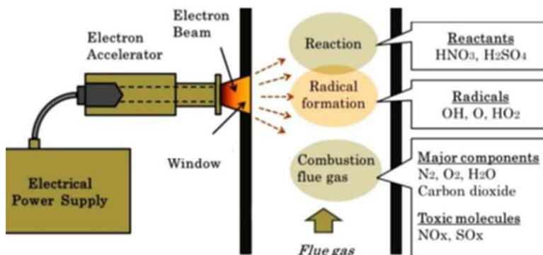
Fig.12. Mechanism of electrons interaction with flue gas molecules.
