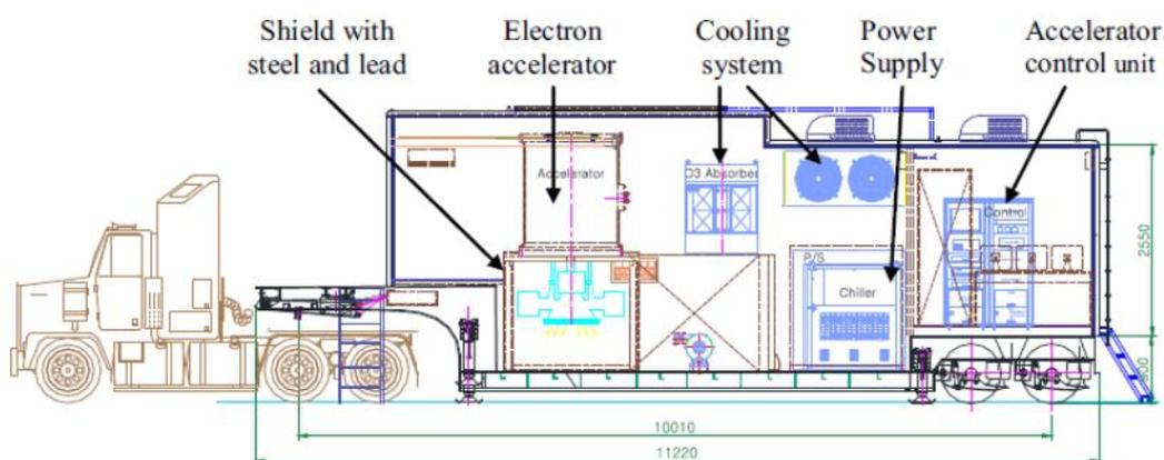
Fig.11b.Mobile EB plant (0.7 MeV, 20 kW), mounted on a trailer.
