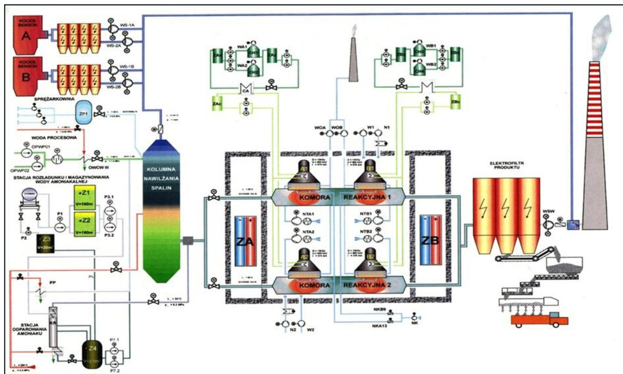
Fig. 7 General layout of the installation.
