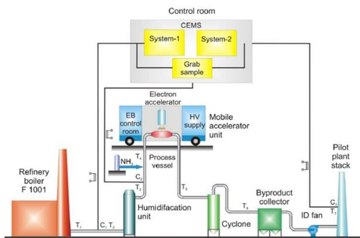
Fig.11a. Layout of pilot plant at the Jiddah Refinery for the electron beam treatment of heavy fuel oil burned flue gas. Not to scale.
