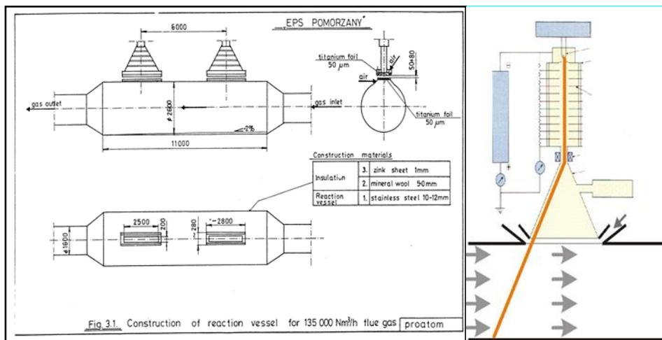
Fig.10. Process vessel cross section (left) and scheme of beam scanning along the gas flow.
