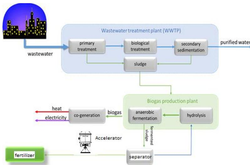
Fig.18. “Zero energy” sludge hygienization technology principle.
