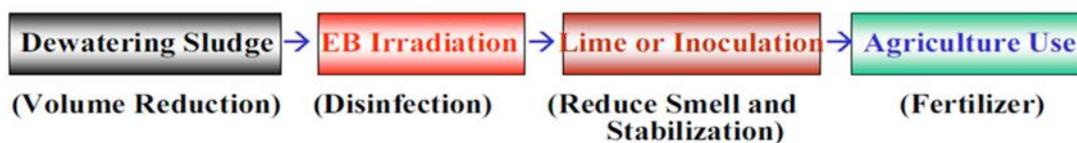
Fig.19 Bio- fertilizer preparation line based on electron beam sludge hygienization.
