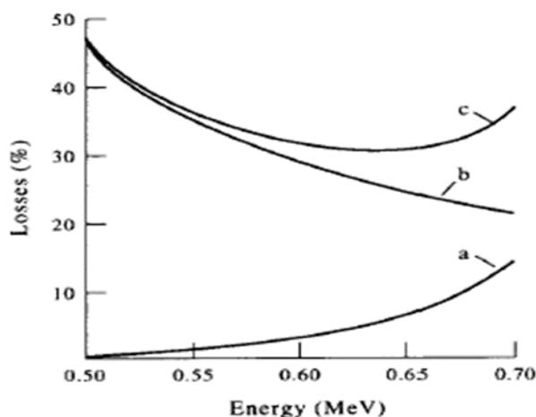
Fig. 5 Energy losses vs. electron beam energy (a-bottom wall, b-windows foil, c-total).
