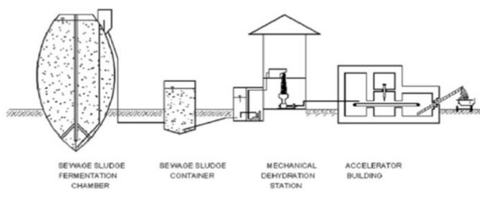
Fig.17 Concept of sludge hygienisation plant with 10 MeV, 10 kW accelerator.
