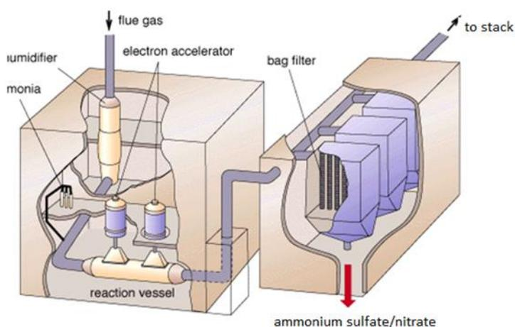
Fig.2 Scheme of EBFGT pilot plant.
