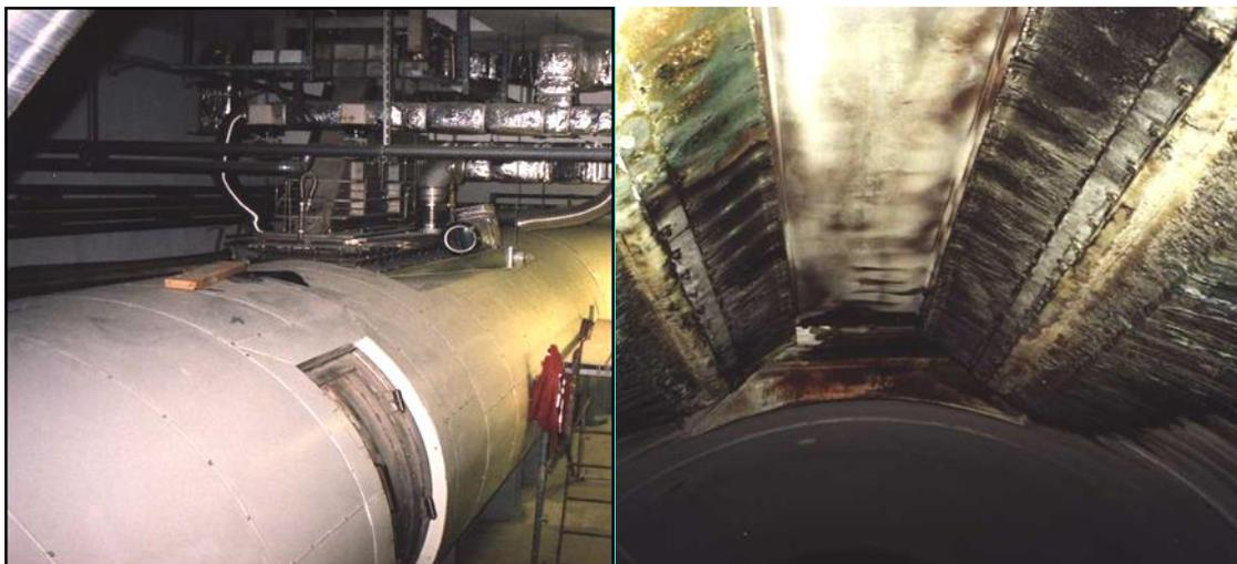
Fig.8. View of process vessel with installed scanning horn (left) and view of titanium window from inside of the flow system ( right).
