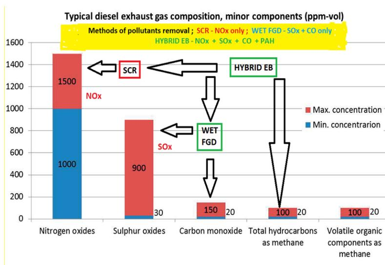
Fig.15. Typical pollutants emission from a marine diesel and methods for their removal.
