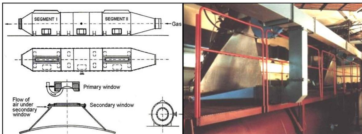
Fig. 4 Cross section of process vessel (left) and view of two scanning accelerator horns mounted on the top of it (right).
