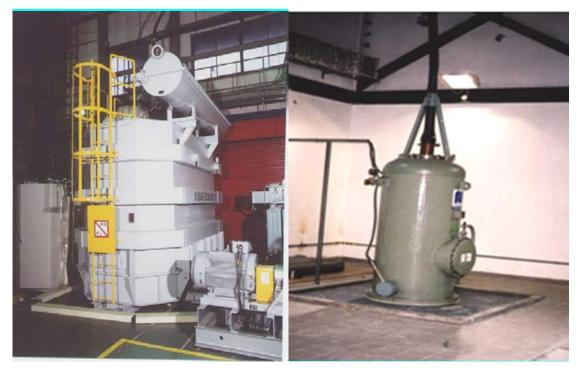
Fig.9. View of the high power supply (total number two) - left and accelerator head ( total number four) - right.
