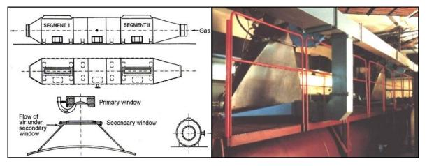
Fig. 4 Cross section of process vessel (left) and view of two scanning accelerator horns mounted on the top of it (right).
