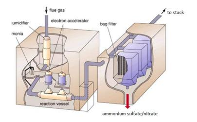
Fig.2 Scheme of EBFGT pilot plant.
