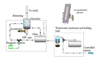
Fig.14 Arrangements of the process units of the hybrid technology for marine diesel of gases treatment.
