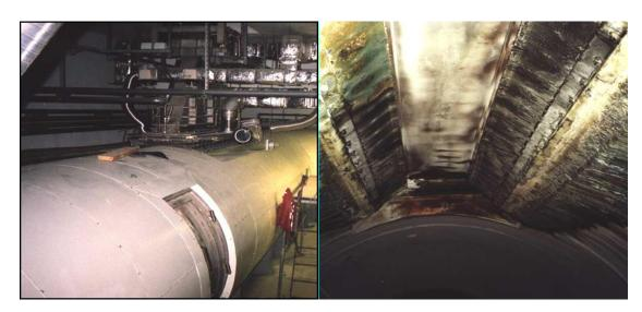
Fig.8. View of process vessel with installed scanning horn (left) and view of titanium window from inside of the flow system ( right).
