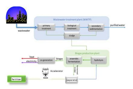
Fig.18. "Zero energy" sludge hygenization technology principle.
