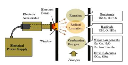
Fig.12. Mechanism of electrons interaction with flue gas molecules.
