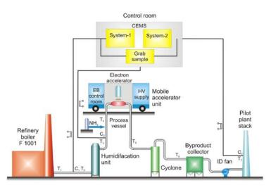
Fig.11a. Layout of pilot plant at the Jiddah Refinery for the electron beam treatment of heavy fuel oil burned flue gas. Not to scale.
