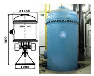
Fig.3 The view of accelerator ELV-3a applied at the pilot plant (two units installed).
