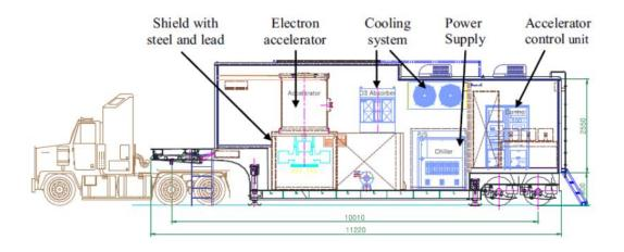
Fig.11b.Mobile EB plant (0.7 MeV, 20 kW), mounted on a trailer.
