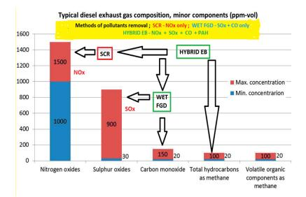
Fig.15. Typical pollutants emission from a marine diesel and methods for their removal.
