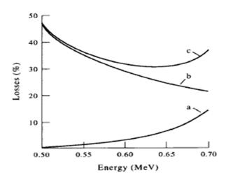
Fig. 5 Energy losses vs. electron beam energy (a-bottom wall, b-windows foil, c-total).
