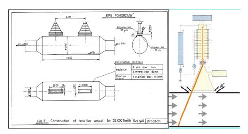
Fig.10. Process vessel cross section (left) and scheme of beam scanning along the gas flow.
