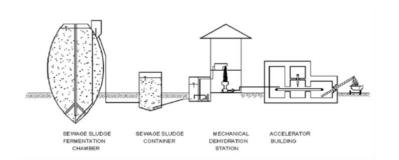
Fig.17 Concept of sludge hygenisation plant with 10 MeV, 10 kW accelerator.
