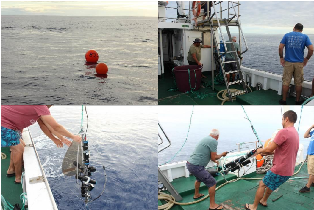
Figure 49 Images taken during the recovery of the Azor drift-cam after getting entangled the previous day. The buoys were used to mark the position of the umbilical when left underwater overnight.
