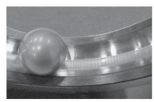
Fig. 1-11 – Bearing race with fluting patterns [22]
