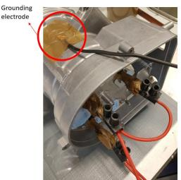
Fig. 4-11 - Auxiliary cabling connection for the CM in the e-ACC machine
