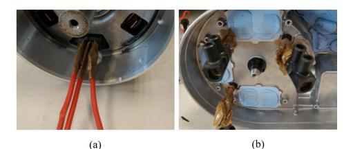
Fig. 4-10 - Machine terminal interface detail, (a) e-PS, (b) e-ACC
