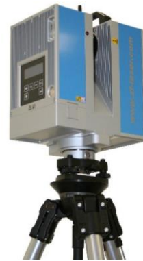
Figure 6. Z+F 5006i laser scanner
