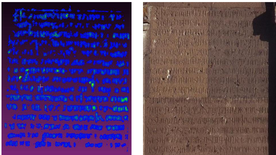
Figure 11. TLS (Z+F 5006i) Data according to new approach values (Left) and original point cloud (Right, URL 3)
