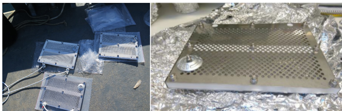
Figure 2.4.1: Deployment cages for passive samplers used on the INTAROS moorings.
