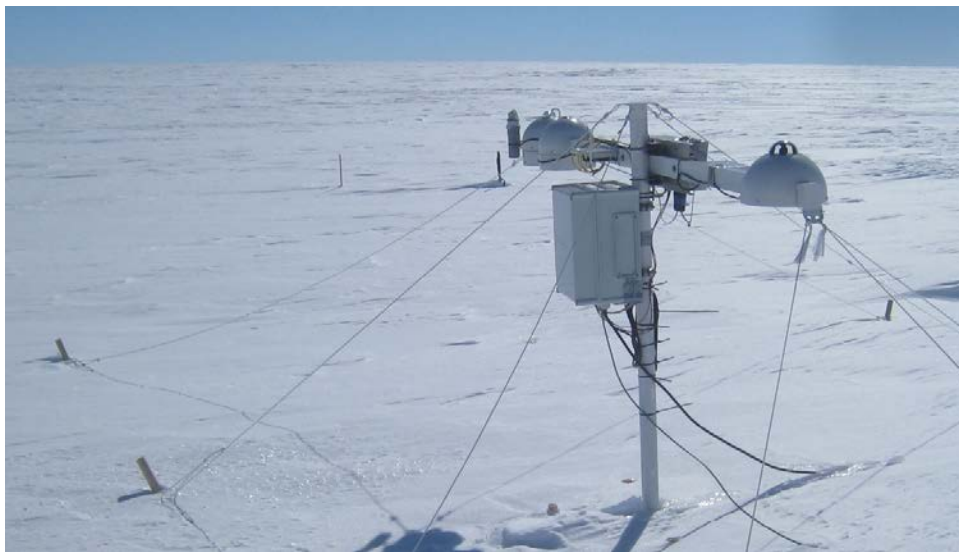
Figure 2.2.2. FMI broadband radiation station installed over the MOSAiC drifting ice floe.
