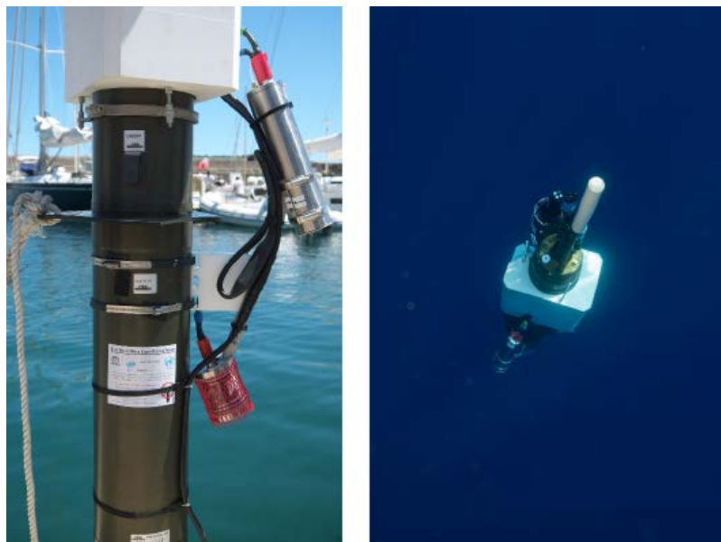
Figure 2.5.2 Proice Argo float equipped with an UVP6- (picture courtesy LOV2).
