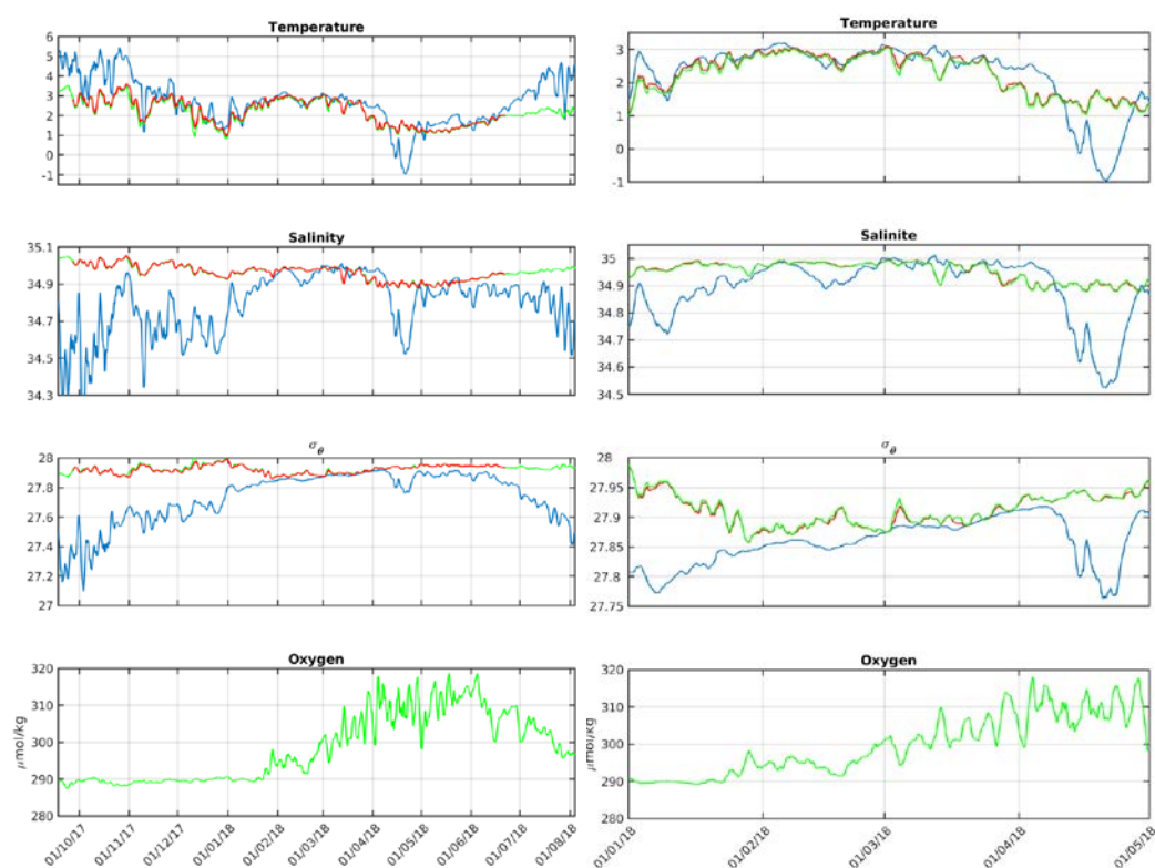
Figure 2.7.2: Time series of temperature ( ^{\circ}\text{C} ), salinity, potential density referred to surface (in sigma units) and dissolved oxygen concentration ( \mu\text{mol/kg} ) as a function of time at about 30 m (blue) and 500 m (green at CNRS1, red at CNRS2) over the period (left) 16/09/2017-3/08/2018 and (right) 01/01-01/05/2018. Data have been smoothed with a 2-day moving average. Note that values have not been corrected for instrument depth changes due to vertical excursions of the mooring line.
