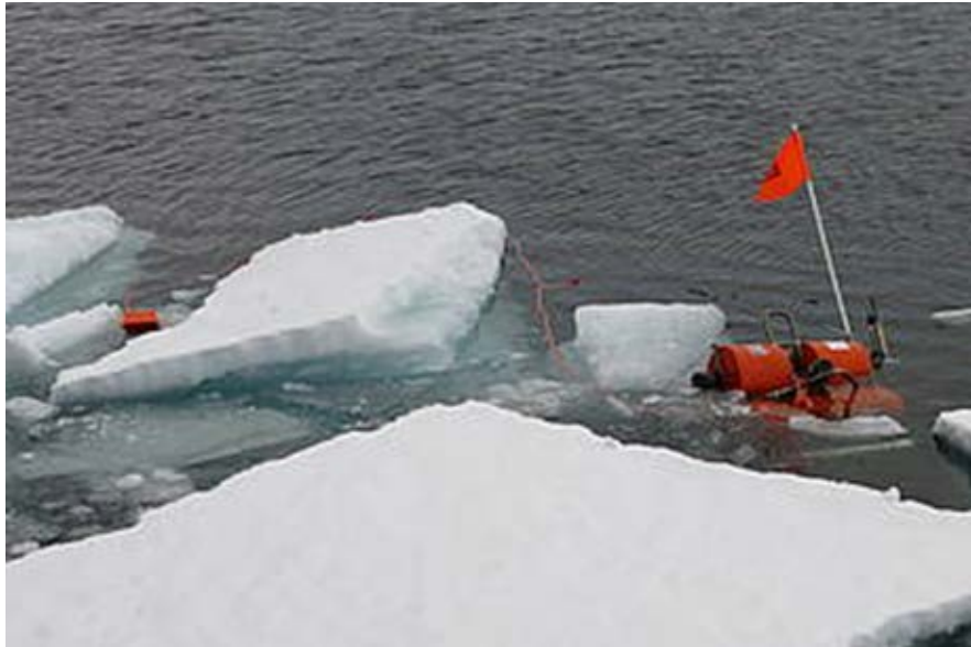
Figure 2.9.4: An OBS instrument surfaced close to a sheet of ice. (Photo: Thomas Funck)
