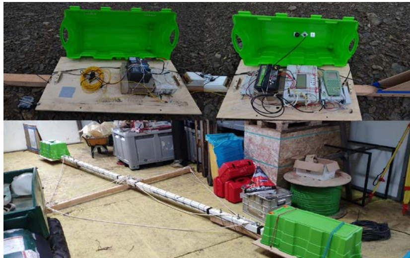
Figure 2.4.1. GPR system deployed in the Antarctic Campaign 2018-19 in Livingston Island, Antarctica: transmitter (upper, left panel), receiver (upper, right panel) and wooden frame (lower panel) for transportation of the radar system hanging under a helicopter. The wooden frame holds the transmitter and receiver subsystems in the green boxes and the transmitting and receiving antennas along the main arm of the frame.
