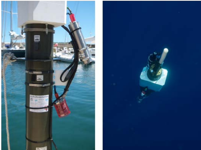
Figure 2.6.1. Proice float equipped with an UVP6- picture courtesy LOV.
