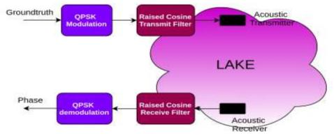
Fig no. 3:- Alternative Acoustics underwater Communication Channel.
