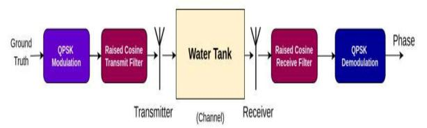
Fig no 2:- An overview on underwater Communication Channel.
