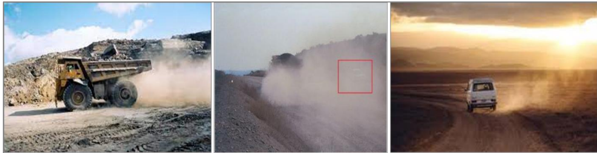
Fig. 3 Left: Example of haul road dust from mine haul tracks, Middle: Light fleet vehicle in the red outline showing the degree of obstruction from dusty haul rods and Right: Dust from an unpaved road
