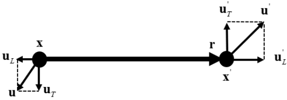
Figure 3. Sketch of longitudinal and transverse velocities, where \mathbf{u}_T and \mathbf{u}'_T are transverse velocities at two locations \mathbf{x} and \mathbf{x}' . u_L and u'_L are two longitudinal velocities.
