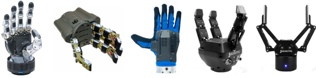
Fig. 3. All the tested end-effectors (in simulation and/or with real hardware) from left to right: SCHUNK SVH, HERI II, qb SoftHand, Robotiq 3F, Robotiq 2F-140.
