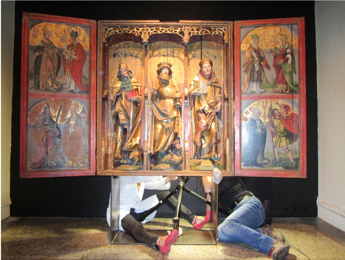
Fig. 3. Kvæfjord 1 altarpiece. Attaining macro photographs of the tree-rings of the altarpiece in the museum exhibition. Three people are occupied here, one to hold the lamp at an oblique angle, one to hold a ruler for scale and one to take the photograph series.
