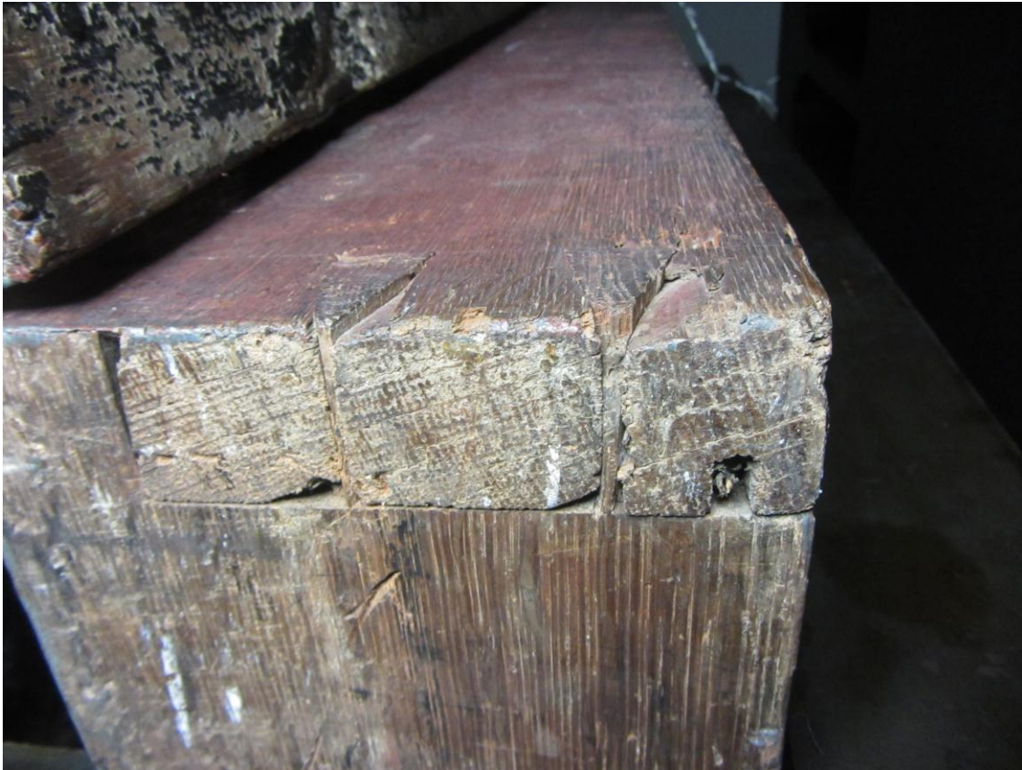
Fig. 4. Kvæfjord 1 altarpiece. Tree-rings on one of the side planks (P7) were measured from the transverse section exposed at the corner dovetail joint.
