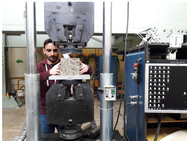
Figure 6: Compression test setup
