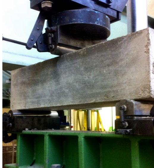
Figure 13: Bending tensile test setup
