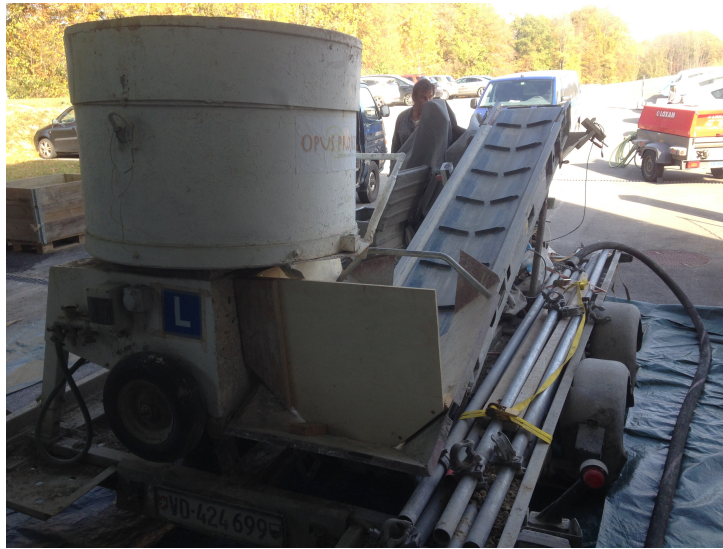
(a) Boulder Gun machine used for spraying
