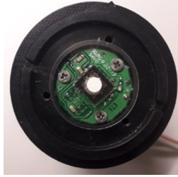
Figure 4: Photo of a 0.5 mm thick specimen coupled to the SiPM.
