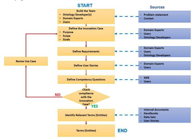
Figure 7: How to start an Ontology module development project
