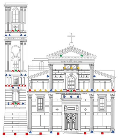
Figure 16. The position of the Luminaires on the main façade and belfry
