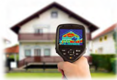
Figure 5. THERMAL CAMERAS Examine non destructively the hidden historical elements in the building's fabric. Detect various threats Differentiate building materials. (Brooke, 2018) (Hendriks, 2019)
