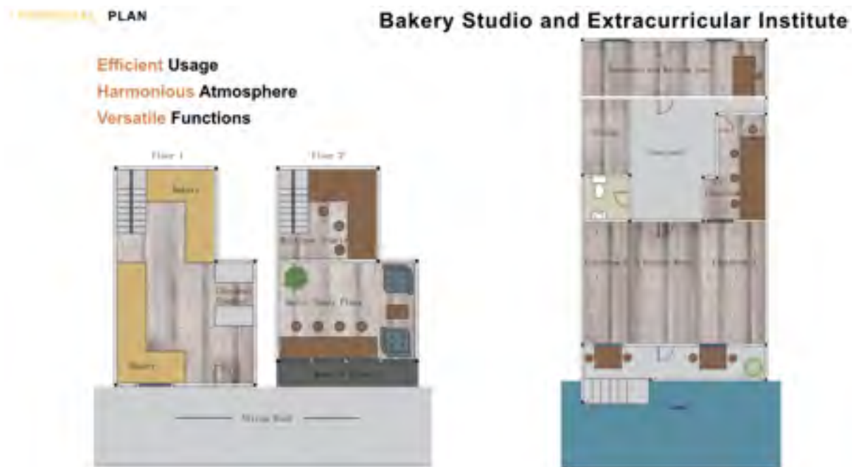
Figure 8. Examples of restructuring the interior of Xixing's traditional houses for modern usages that improve functions. Drawn by the author.
