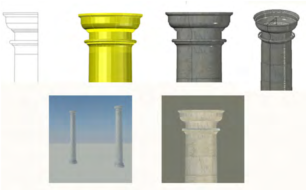
Figure 28. . Direct modelling of a Doric column in Autocad(Author).
