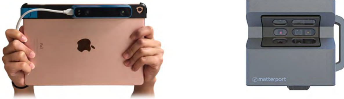
Figure 37. Left : Canvaswith Structure Sensor (CANVAS, 2018) Right : Matterport 3D Camera (Matterport, 2019) .
