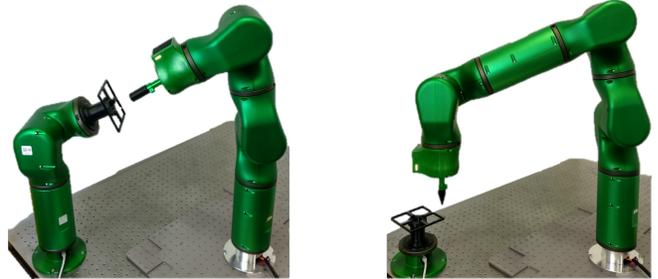
Fig. 1: Two robot configurations for the peg-in-hole (left) and contour-following task (right).
