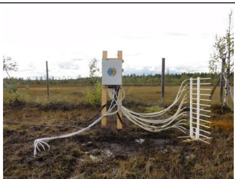
Figure 18. Typical station set-up with soil sensors in the ground and a snow temperature profile.
