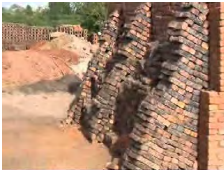
Figure 13. the way to keep blocks together safe in a dynamic environment is to have them on an inclined planes.
