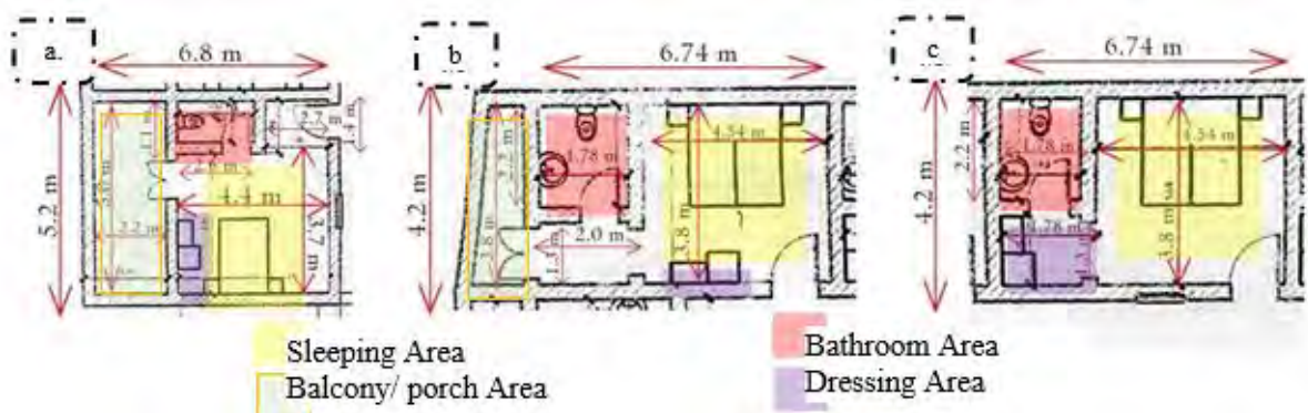
Figure 8. Katoo-doolNubian house rooms layouts, (a)Room size of Standard ecolodge, (b) Room size of Suite ecolodge, (c) Room size of Deluxe ecolodge. (Researcher)
