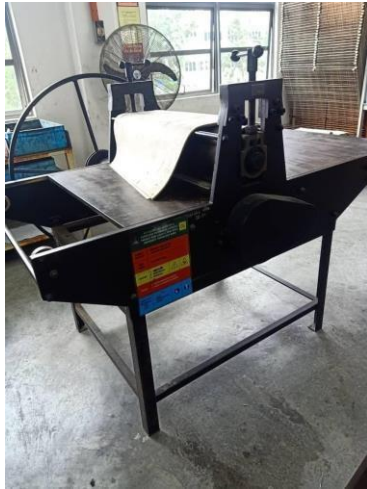
Figure 9. Etching Press Machine used in the conventional process of a Drypoint print. (Source: Researcher)
