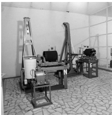
Figure 7 – Mainka Modified seismographs with 540 kg mass (left) and Mainka seismographs with 180 kg mass (right) at the Timișoara seismic station (Source: Timișoara seismic station Archive).
