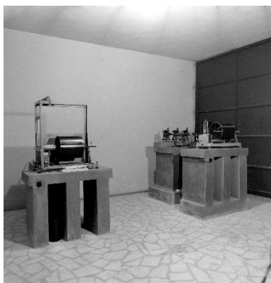
Figure 8 – Vegik Electrodynamic seismographs (left) and Kirnós – SKD (right) at Timișoara seismic station (Source: Timișoara Seismic Station Archive).
