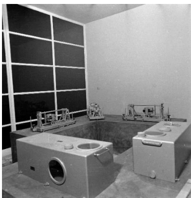
Figure 8 – Vegik Electrodynamic seismographs (left) and Kirnós – SKD (right) at Timișoara seismic station (Source: Timișoara Seismic Station Archive).
