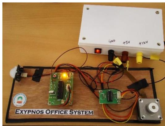
Figure 11. Hardware setup for door entrance system
