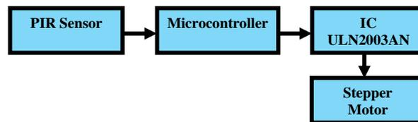
Figure 4. Block diagram of door entrance system
