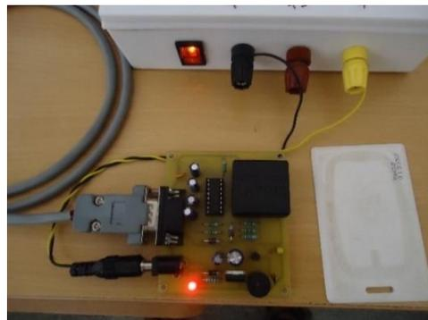
Figure 15. Hardware setup for RFID reader
