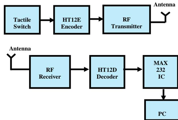
Figure 5. Block diagram of employee system/monitor
