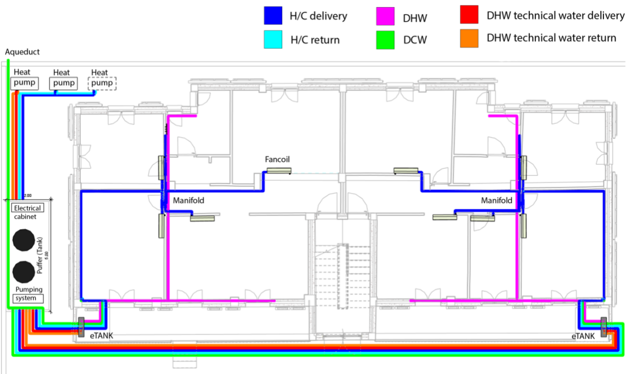
Figure 31: Pipe distribution from the cabinet to the internal units: plan view of a typical floor.
