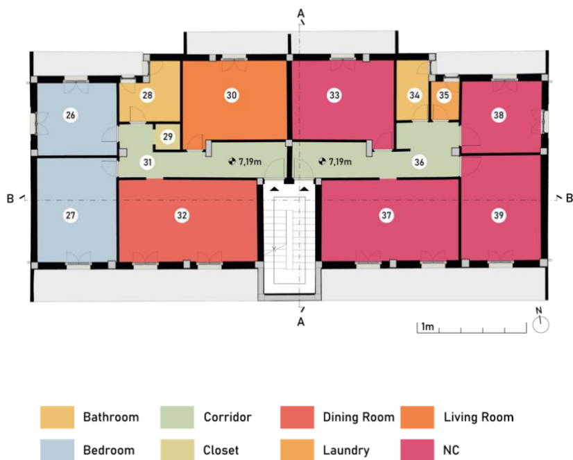
Figure 11: Distribution of apartments on the 2 nd floor.
