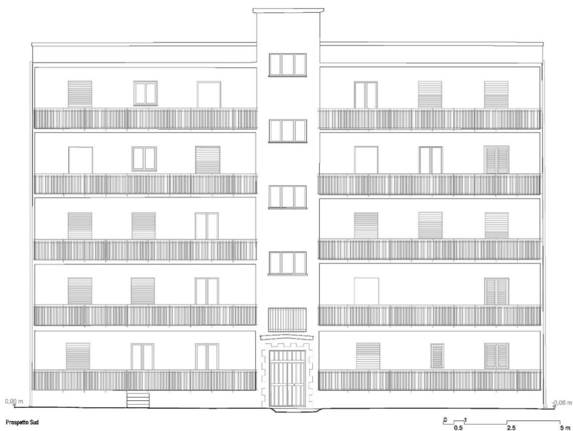
Figure 8: The south front of the pilot building.
