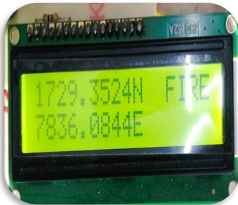
FIG-7 :when fire is detected.
